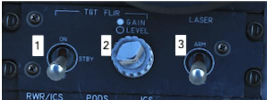
Power to the LANTIRN pod can be initiated only from the back cockpit, using a switch on the Sensor Control Panel (1). The same panel governs the gain / level (2), as well as arming the laser (3).
