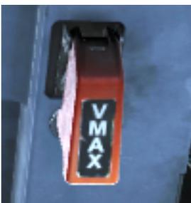
This switch was used in the F-15E with PW-220 engines and has no function with the PW-229.
