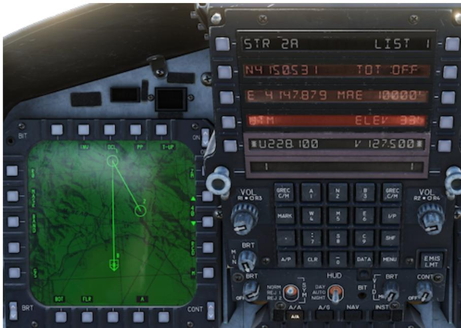
*NOTE: if new Steer Point number typed is higher by 2 or more than the highest SP currently stored in the system, the CC will create the SP with the entered number and not default to next available one. In the case above, if aircrew types 23 as new Steer Point number, it will create SP 23 and not SP 3.*
