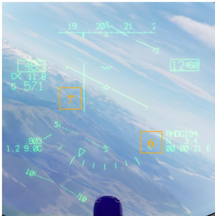
On the HUD, AHDG legend will also be displayed in the NAV data block to signify that the HDG coupled mode is active (6). A vertical steering line will also be shown (7).
