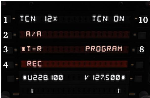
**PB 1:** TCN channel. Pressing this PB switches between X and Y modes.
