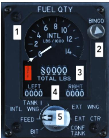
1. Internal Fuel Gauge shows total internal fuel with readings multiplied by 1000.
