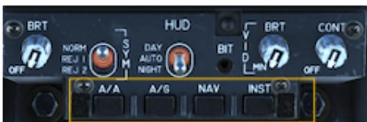
The master modes are selected with the switches below the Hud Control Panel.
