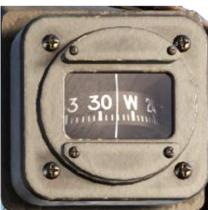
A conventional magnetic compass mounted on the canopy arch. It is available only in the front cockpit.
