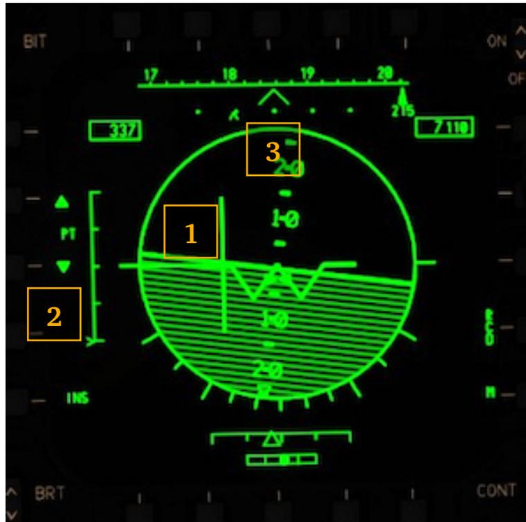
1. The vertical and horizontal bars are superimposed over the artificial horizon and mirror the indications from the HUD.
