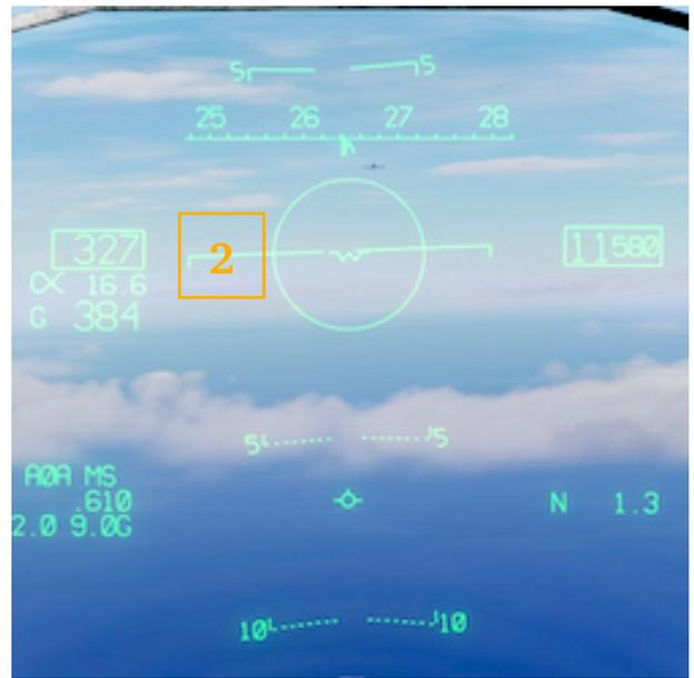
On the radar display, **BST** legend in the bottom - left part (1) indicates that the radar is in Boresight mode. On the HUD, target should be placed in the scan circle to achieve an automatic lockon (2), upon which the radar enters normal STT.
