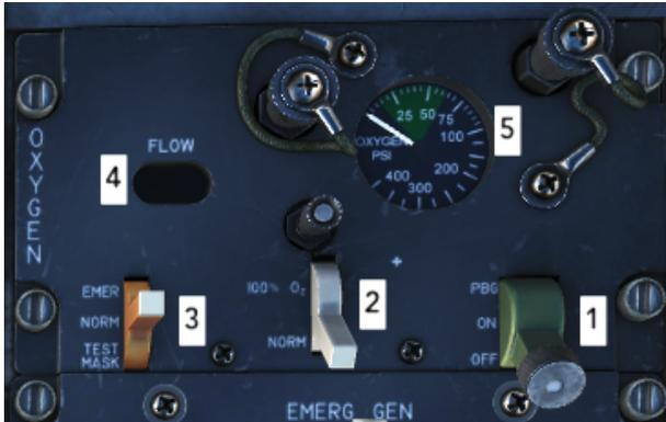
Control panel for the Molecular Sieve Oxygen Generating System (MSOGS). The MSOGS provides a continuously available supply of breathing gas for the aircrew.
