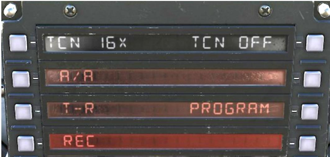
Info next to PB 1 shows the currently selected TACAN channel. To change it, a new number should be entered in the scratchpad. After pressing PB 1, this channel will be set and the TACAN will automatically enter into the T-R mode (marked with asterisk next to it), with TCN ON information displayed next to PB 10.
