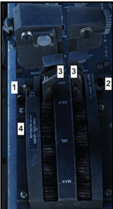
The front throttle quadrant contains the front throttles, finger lifts, friction adjusting lever, rudder trim switch and flap switch. Additionally, the throttle grips contain switches to provide various system controls without moving the left hand from the grips.
