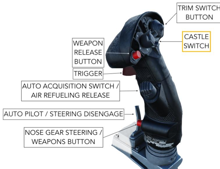
In the front cockpit, the pilot uses LONG PRESS Castle Switch to take command of MPD and SHORT PRESS towards the desired display to scroll between the programmed display formats.
