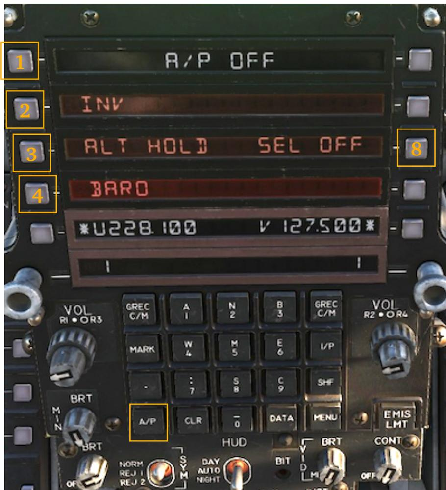
A/P button on the UFC enables or disables the autopilot. Mode entered upon pressing the button depends on several factors, as described below. It also brings up the A/P menu displayed above.
