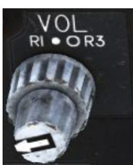
The left Volume Knob controls the volume of UHF radio (R1) with the outer (smaller) knob. The inner (larger) one is used for the second V/UHF radio (R3).
