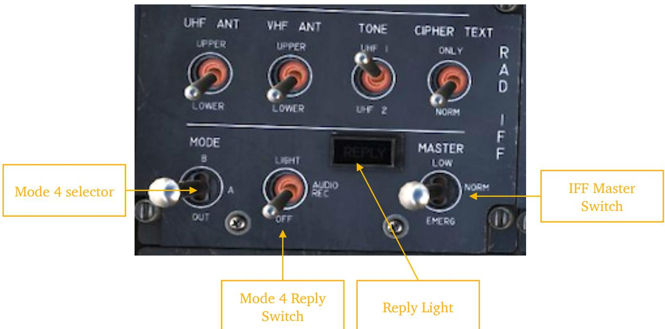
**Mode 4 selector switch for the IFF** has three positions:
