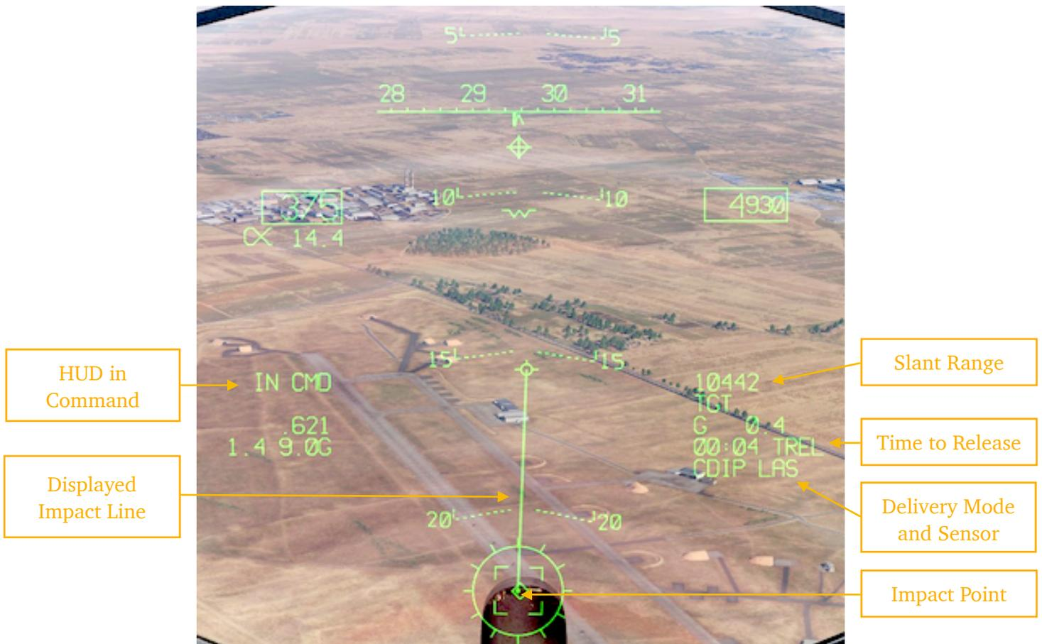
**DISPLAYED IMPACT LINE:** the DIL provides an azimuth steering reference to aid in positioning the reticle on the target. It is limited to the edge of the reticle to allow clearer viewing of objects in the reticle.
