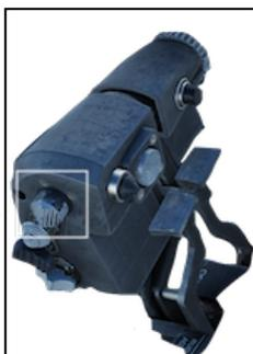
A three-position Microphone Switch on the right throttle in each cockpit governs the UHF and V/UHF transmission. It is spring-loaded to the center (receive) position.
