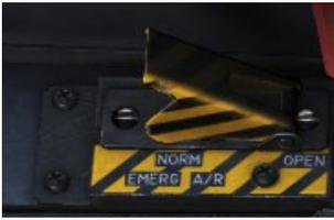
It can be used to open the AAR slipway door by the means of pyrotechnic devices. However, that means that the door cannot be then closed in flight. However, if set to “CLOSE”, it will still restore the pressurization of the external fuel tank.
