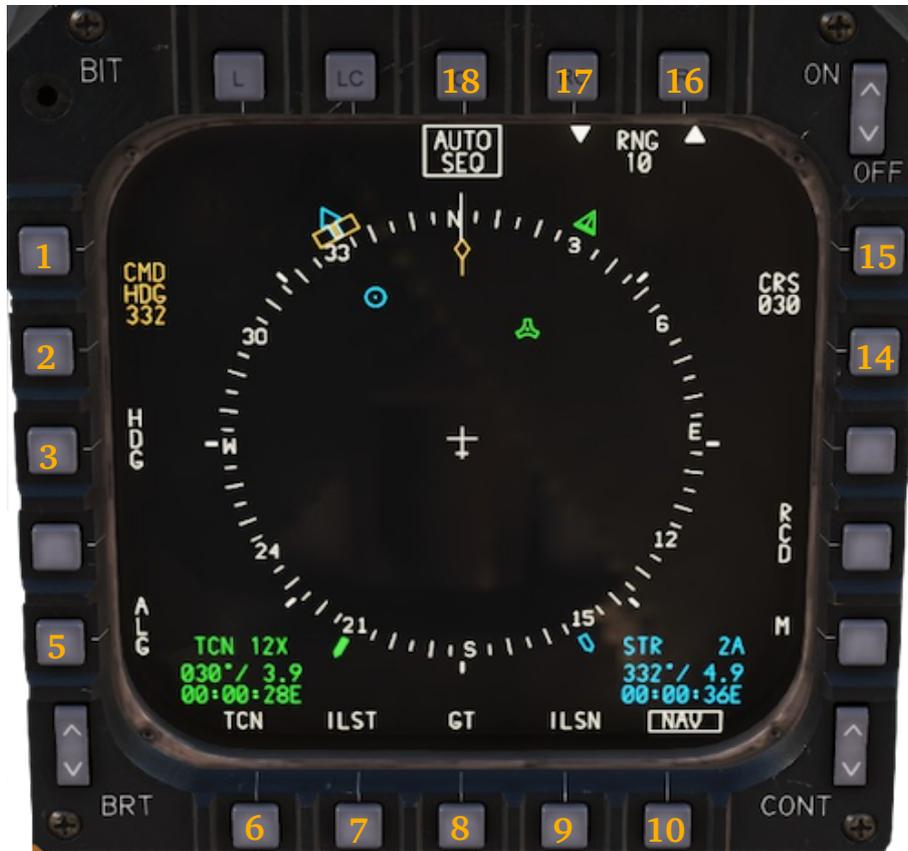
**PB 1 - 2, CMD HDG:** used to move around the command heading marker. PB 1 increases the value by one with each press, PB 2 decreases it. Desired heading can also be typed in the scratchpad and then entered by pressing either of the two PBs. In NAV mode the marker is coupled with the NAV bearing pointer, and the CMD HDG field displays the heading towards the selected Steer Point (which corresponds to information visible in the second line of the NAV Data Block).
