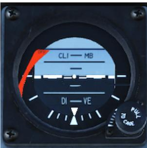
**Standby Attitude Indicator** is a self-contained, electrically driven gyro-horizon type instrument. If there is no power or the gyro is caged, the OFF flag appears. In order to uncage the gyro, the pilot should pull the knob. The indicator displays rolls through 360 degrees, climb up to 90 and descend down to 78 degrees.
