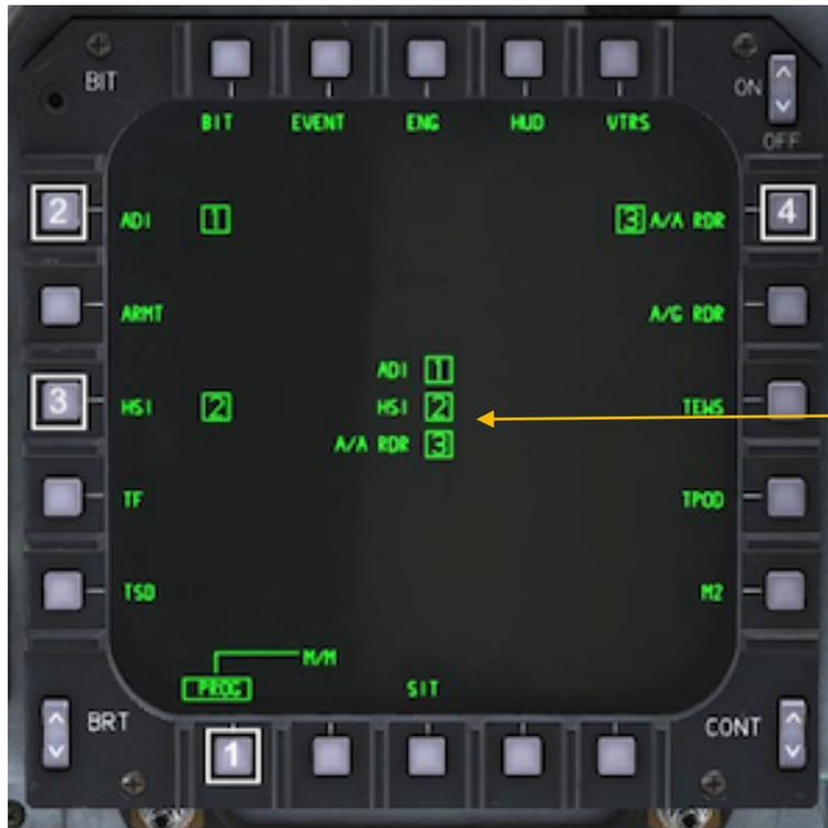
Program the displays for the selected MPD / MPCD as described in previous section.
