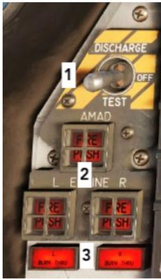
1. Fire Test / Extinguisher Switch has three positions:
