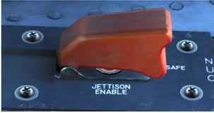
This guarded switch is exactly the same is in front cockpit. It allows the crew to release or jettison nuclear weapons onboard. Three positions: SAFE, RELEASE and JETTISON ENABLE. Both switches have to enabled for RELEASE or JETTISON.
