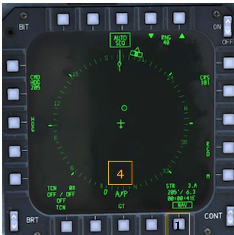
Second line of display on the UFC will show **STR MODE-NAV** legend with an asterisk next to it (2). When the A/P button is pushed on the UFC, **A/P NAV** shows in the first line of display (3), with additional **A/P** information on the HSI (4).
