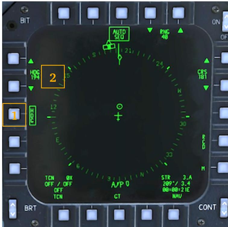
On the HSI, **HDC** should be boxed by pressing PB 3 (1). Desired heading should be selected by using PBs 1 and 2 or by typing the value in the scratchpad and pressing either of these PBs (2).
