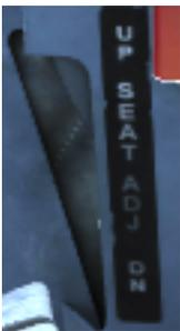
The switch has the three positions of UP and DN and is spring-loaded to the centre OFF position. Maximum vertical seat travel is 5 inches. The seat adjustment actuator does not cut off power to the electric motor at either limit of travel. Release the seat adjust switch when the seat reaches an upper or lower limit to prevent damage to the actuator motor.
