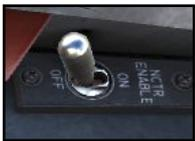
NCTR Auto Enable Switch in ON position enables the auto NCTR entry.
