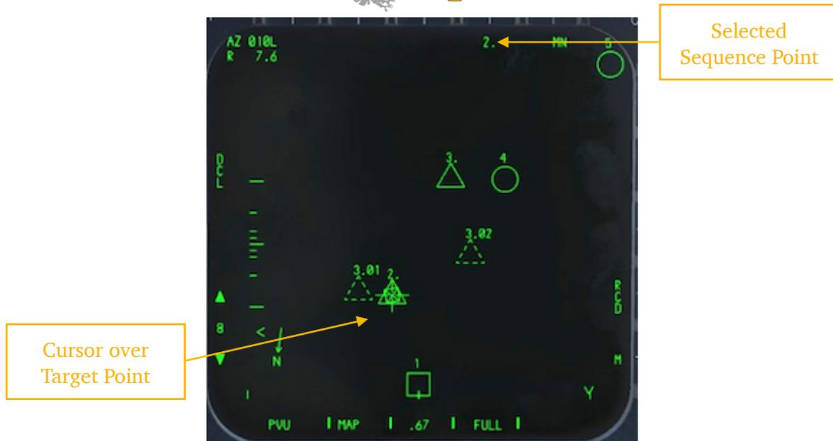
If the selected SP is beyond the radar range the cursor will be limited to the edge of display along the radial from the aircraft to the reference sequence point.
