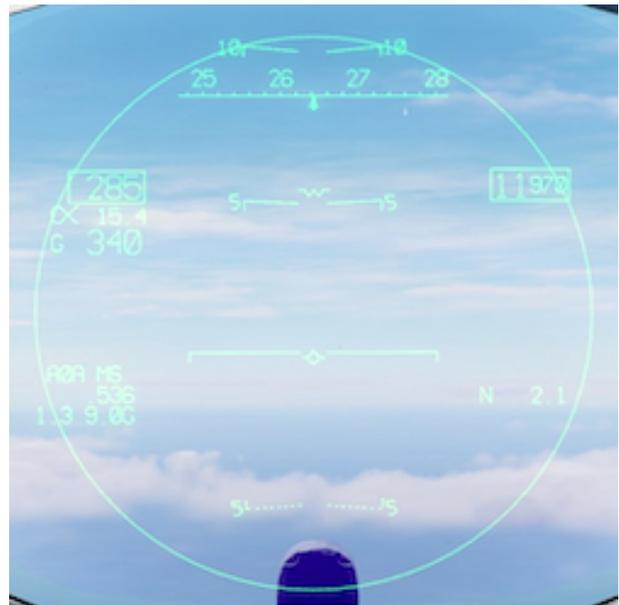
On the radar display, **55** legend in the bottom - left part (1) indicates that the radar is in supersearch. The number before it shows current bar (between 1 and 6), mirrored by the movement of the caret on the elevation scale (2).
