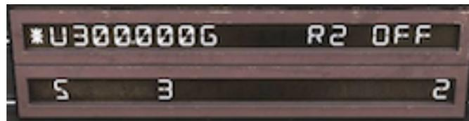
LCD Line 5 displays the manually entered frequency for the UHF radio on the left and the V/UHF radio on the right. The  $\mathfrak{G}$  behind the frequency indicates that Guard monitoring is enabled.
