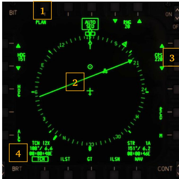
1. In order to enable the PLAN mode, with TCN boxed press PB 20.
