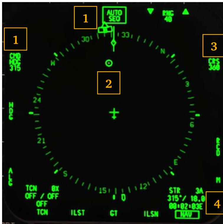
1. Command Heading is displayed next to PB 1 and 2, as well as on the compass rose.
