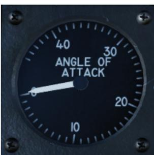
**Angle of Attack Indicator** is only available in the front cockpit and displays indicated AoA in units from 0 to 45. A T shaped index mark show optimum landing approach AoA (between 20 and 22 units). An OFF flag is displayed is there is no power supply for the indicator.
