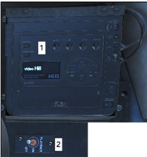
1. The 8mm colour video recorder is capable of recording up to 5 hours of MPD, MPCD and HUD video, together with audio communication to and from the air crew.
