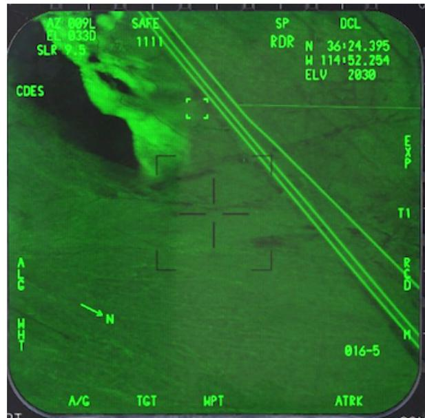
The picture on the left shows the A/G radar in RBM mode. The CUE cursor was selected and spot underneath it was designated (indicated by the **CUE** legend next to it).
