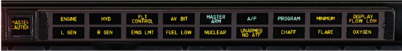
**MASTER CAUTION:** Master Caution Light come simultaneously with any MPD/MPCD caution, as well as all yellow caution lights except PROGRAM, MINIMUM, CHAFF, FLARE, LOCK/SHOOT, AV BIT, LASER ARMED, EMIS LMT and UNARMED/NO ATF. Pressing the Master Caution makes the MASTER CAUTION lights in both cockpits go out, except for the AUTO PLT caution (it remains on until the malfunction is corrected).
