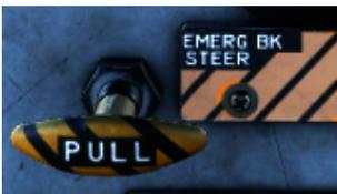
When pulled, this handle provides additional power from JFS hydraulic accumulator to the brake system and for the nose gear steering. In case of brake failure, sufficient power is provided to safely stop the aircraft.
