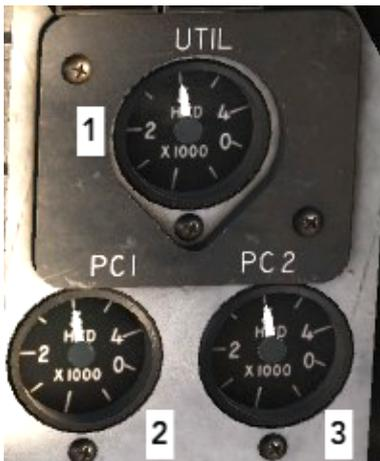
1. Utility Hydraulic System Pressure Gauge monitors the operation of two pumps: left with pressure of 3000 psi and right with pressure of 2775 psi.
