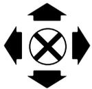
A four - way switch (FWD - AFT - LEFT - RIGHT) spring-loaded to center (neutral) position.
