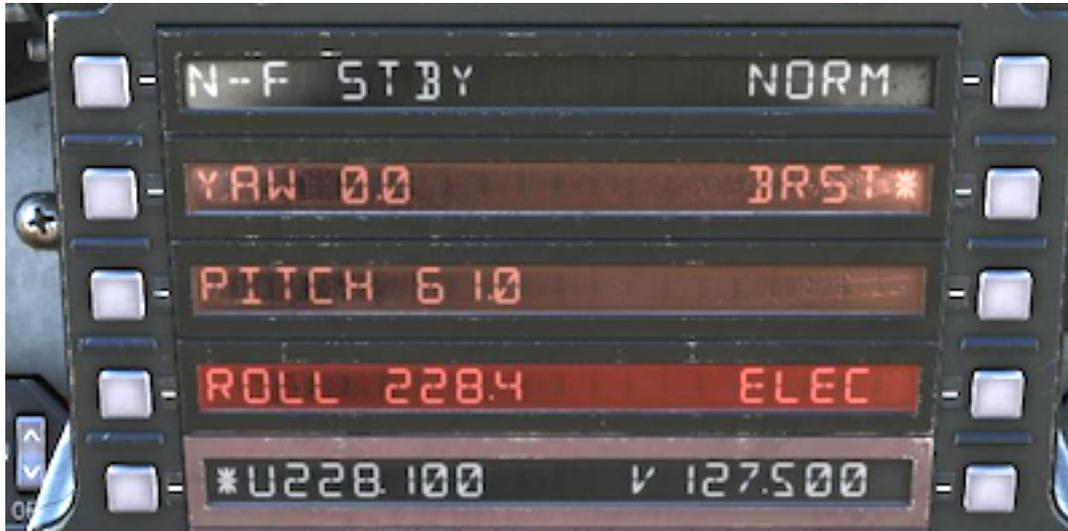
In the real aircraft, the values indicated next to YAW (PB 2), PITCH (PB 3) and ROLL (PB 4) should agree with the unique mechanical boresight numbers stored in CC and also listed on a special form available to the aircrew.
