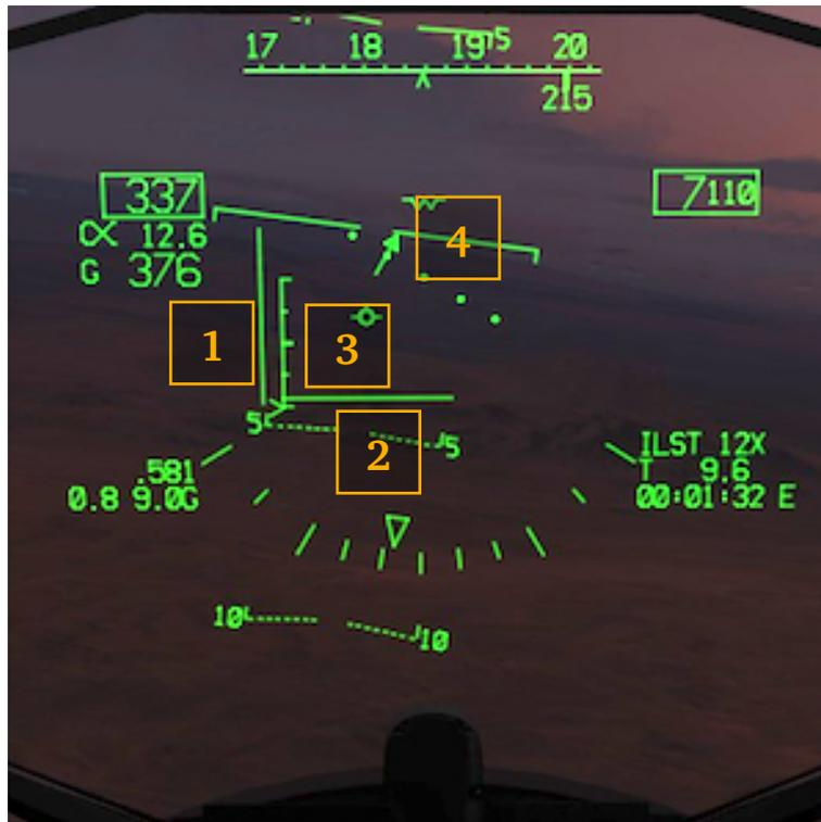
1. The ILS localiser vertical and horizontal (2) bars indicate the position of the aircraft in relation to the glideslope. They are not tied to the TACAN or Steer Point, but are based on the indications from the ILS localiser.
