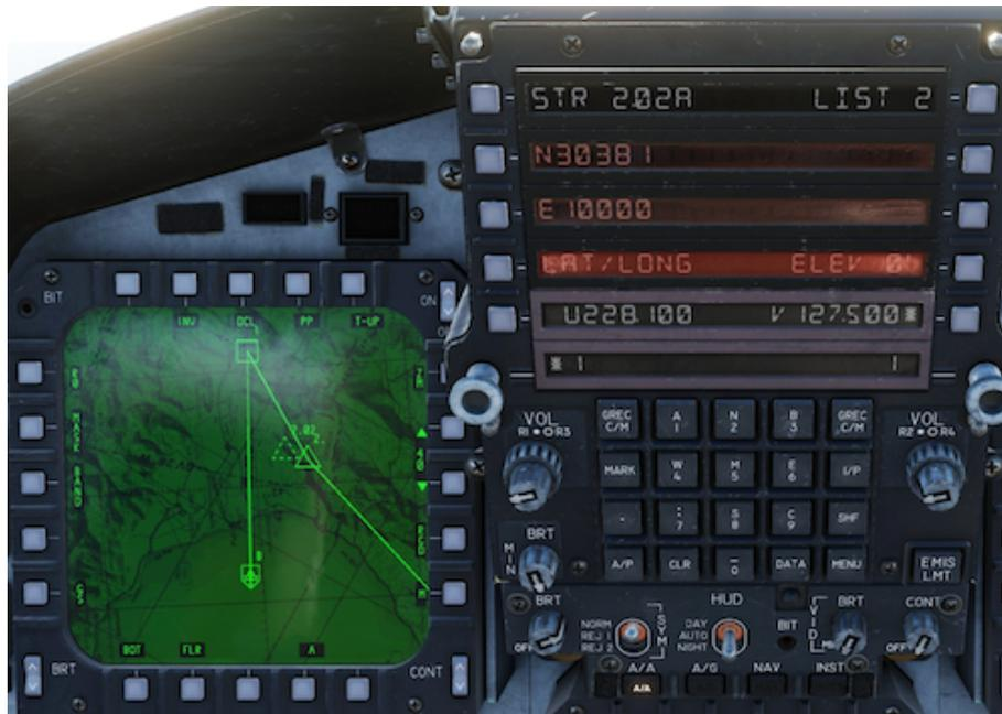
To create a new Offset / Aim Point using this system, a cardinal N-S and E-W direction should be determined first.
