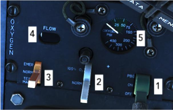
Control panel for the Molecular Sieve Oxygen Generating System (MSOGS) is exactly the same in the back seat as in the front. The MSOGS provides a continuously available supply of breathing gas for the aircrew.
