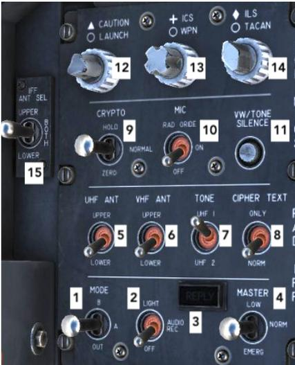
Contains controls for the IFF transponder set, VHF, UHF and Intercom controls as well as volume knobs for different systems.
