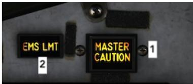
1. Master Caution Light come on simultaneously with any MPD/MPCD caution, as well as all yellow caution lights except PROGRAM, MINIMUM, CHAFF, FLARE, LOCK/SHOOT, AV BIT (Avionics BIT), LASER ARMED, EMIS LMT and UNARMED/NO ATF (Automatic Terrain Following).
