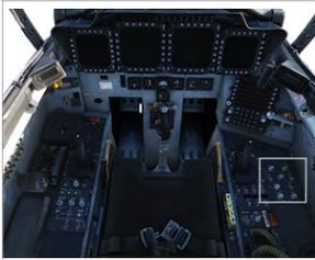
Press the **Lights Test** switch (3) and check if all the warning and caution lights function properly.
