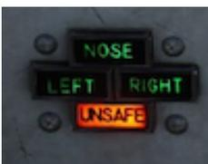
Landing Gear Position Lights are marked NOSE, LEFT and RIGHT. Each of the lights illuminates when when its respective gear strut is down and locked. There also is an UNSAFE indication, which lights up whenever any landing gear is not locked in the commanded position.
