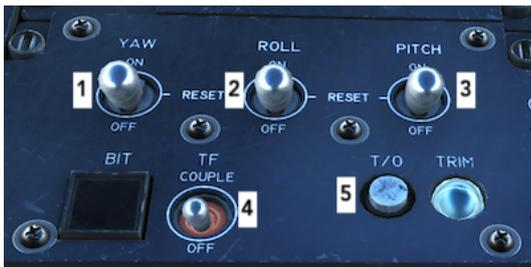
1. YAW CAS 3-position switch. ON allows normal operation after engagement, RESET engages disconnected axis after the fault that caused the disconnect no longer exists (it is spring loaded back to ON), OFF disengages the applicable axis.
