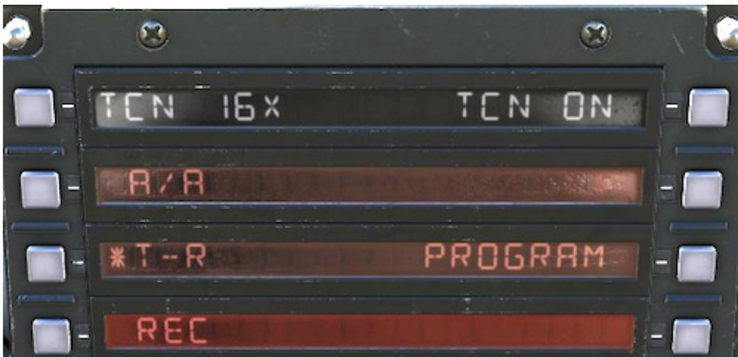
Pressing the PB 8 (PROGRAM) opens another page which allows to enter additional data for the TACAN station.
