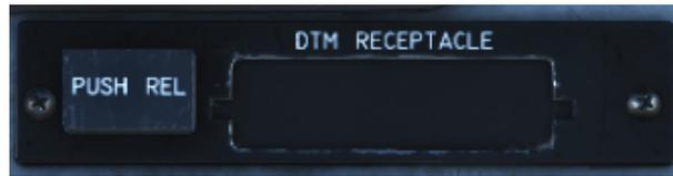
The DTM consists of the DTM Receptacle (DTMR) on the main instrument panel and the Data Transfer Module (DTM). Mission data is loaded, by the aircrew or operations personnel, on the ground and stored in the module. The module is carried to the aircraft and inserted by the pilot into the DTM receptacle to initialize mission data.
