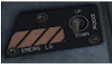
The arresting hook control switch is located on the front and rear cockpit left sub panels. In UP position the hook is retracted. In DOWN position the hook is lowered.
