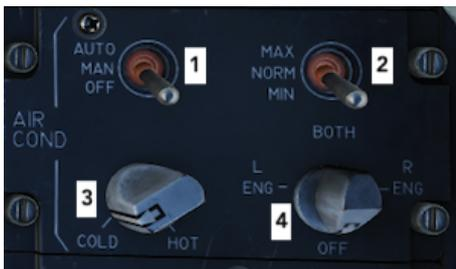
1. Cockpit Temperature Switch. Controls internal temperature. Three positions: AUTO, MANUAL and OFF.
