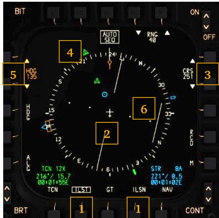
1. In order to enable the ILST or ILSN mode, PB 7 or PB 9 should be pressed, respectively. The selected steering mode becomes boxed.
