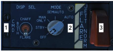
The CMD control panel applies CMD operations power, selection of payload dispensing modes, and selection of flare jettison.
