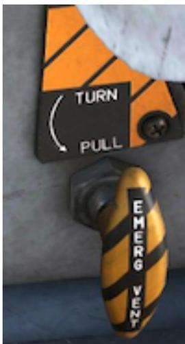
The emergency vent handle electrically dumps cabin pressure when turned 45 degrees counterclockwise. When extended, it shuts off ECS air to the cockpit and allows ram air to enter.
