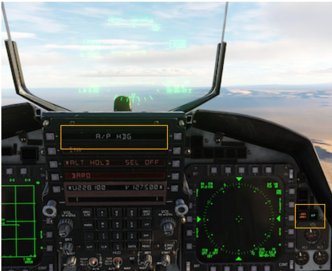
The currently selected mode will be displayed in the top line of the UFC with A/P submenu or on MENU 1 page next to PB 9. Additionally, a green **A/P** light will come on on the caution panel next to the right MPD.
