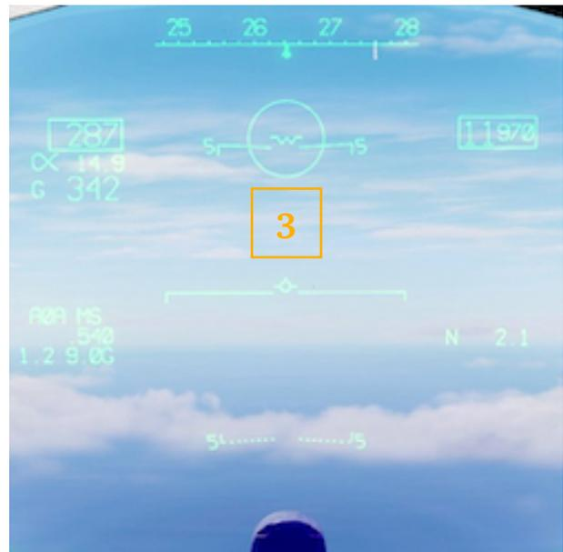
On the radar display, **LR BST** is displayed in the bottom - left part (1). The range of the scan is set to 40 NM (2). On the HUD, target should be placed in the scan circle to achieve an automatic lockon (3), upon which the radar enters normal STT.
