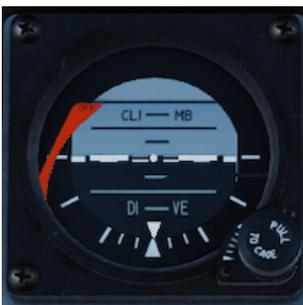
**Standby Attitude Indicator** is a self-contained, electrically driven gyro-horizon type instrument. If there is no power or the gyro is caged, the OFF flag appears. In order to uncage the gyro, the pilot should pull the knob, rotate and then release. The indicator displays rolls through 360 degrees, climb up to 90 and descend down to 78 degrees.
