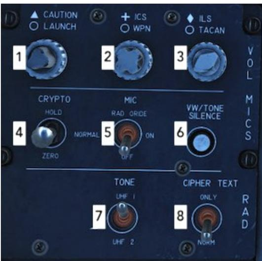
1. Tactical Electronic Warfare System Volume Knob. The top knob is used to set the volume of caution sounds, the bottom (larger) one controls the launch warning volume.
