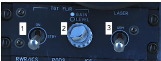
Laser Arm Switch is on the right side of the Sensor Control Panel in the rear cockpit (3).
