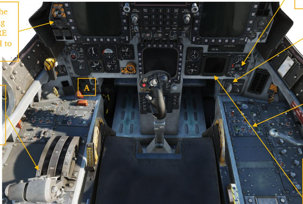
18. Check the fire warning system (FIRE EXT SWITCH to TEST)
