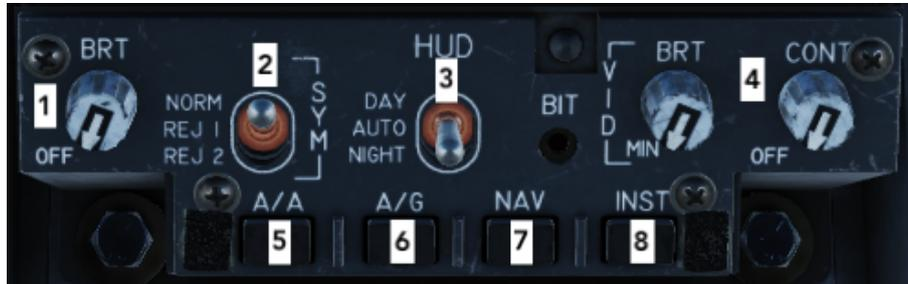
1. Symbol Brightness knob controls the brightness of the HUD stroke symbology. Rotating it clockwise applies power to the HUD.
