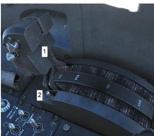
The throttle in the back seat has many less options than the one in the front, because most of the switches have been moved to the Hand Controllers. More information about the functions of the buttons on the throttle (1) can be found in later section of this chapter.
