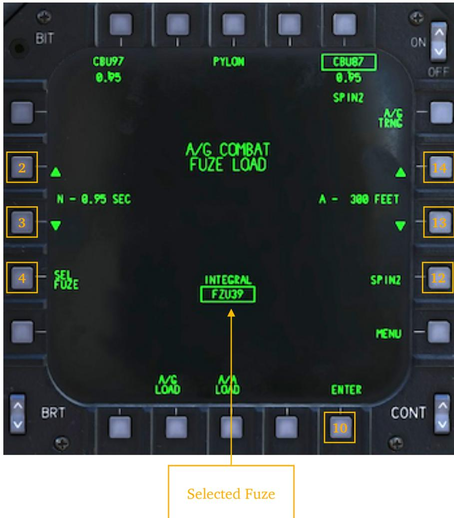
**PB 2-3, BURST TIME:** sets the time from bomb drop in seconds after which the bomblets will be released. There are 11 options available:
