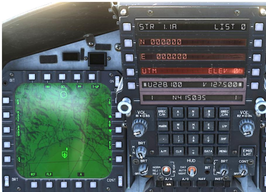
It is possible to create Offset / Aim Points by entering the Lat - Long or UTM coordinates in exactly the same way as for the Steer Points. However, there is additional option available after pressing the PB 4 when in UTM sub-menu (marked RNG / BRG):
