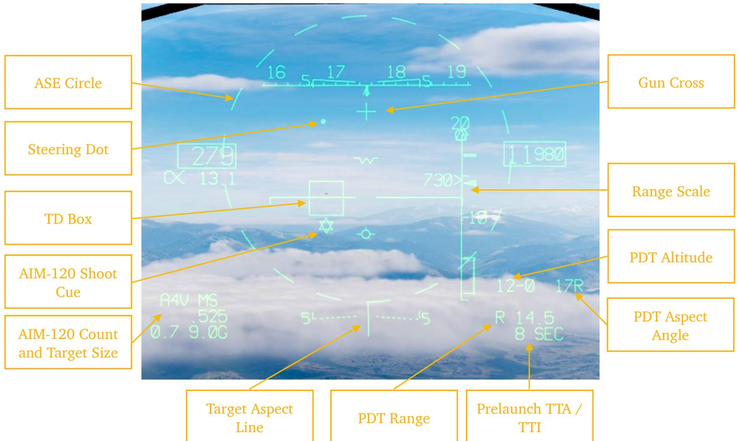
**ASE CIRCLE:** ASE stands for “Allowable Steering Error”. The size of this circle depends on the radar line of sight to the target and missile gimbal limits, which means that it will change depending on these two factors.
