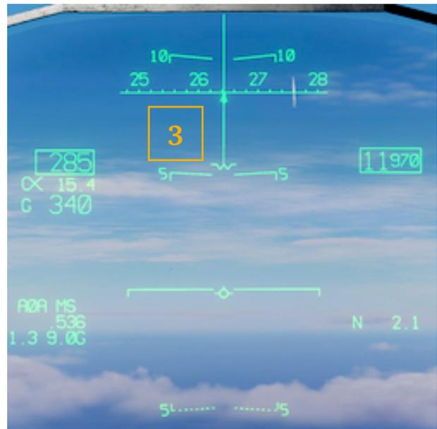
Just like in SS, **VTS** legend in the bottom - left part of radar display (1) indicates that the radar is in vertical scan. The number before it shows current bar (between 1 and 6), mirrored by the movement of the caret on the elevation scale (2). On the HUD, a vertical line extends from the Waterline Symbol to signify that the radar is in VTS.
