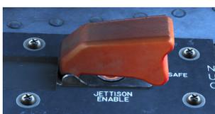
This guarded switch allowing pilot to release or jettison nuclear weapons onboard. Three positions: SAFE, RELEASE and JETTISON ENABLE. The functions of this switch are not implemented.
