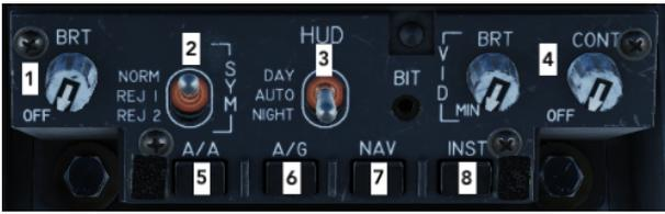
There are two knobs on the HUD Control Panel responsible for the NAV FLIR image displayed on the HUD, namely the **Video Brightness** and **Contrast** (4).
