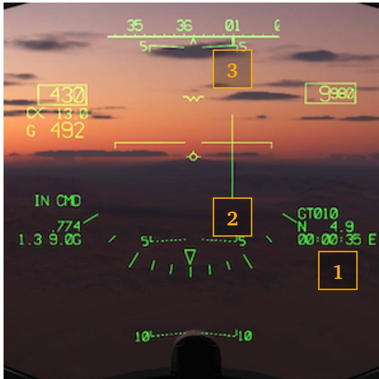
1. On the HUD, GT legend is displayed in NAV data block, followed by the value selected in CRS field on the HSI. Note that the info below still indicates the distance and Time Enroute (or of Arrival) to the currently selected Steer Point.
