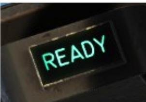
The AR Ready Light indicates that the system is ready for boom engagement. It then goes off once the boom connects and refuelling starts.
