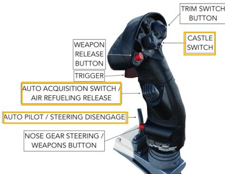
In the front cockpit pilot uses following buttons and switches:
