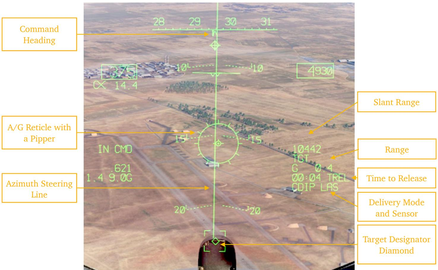
After release, the TREL legend changes into TIMPCT showing weapon time to impact on the HUD, targeting pod display, as well as TEWS and HSI.
