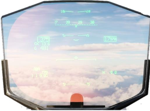
The holographic combiner displays projected raster (video) and stroke (symbols) imagery in a total field of view which measures 21° in elevation and 28° in azimuth. The HUD displays navigation, FLIR video, flight control and weapon delivery information. See [Chapter 6: Head Up Display](#) for more information.
