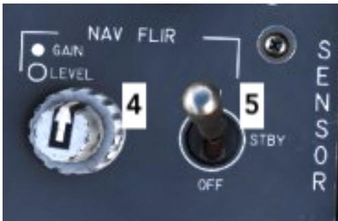
**NAV FLIR Power Switch (5)** needs to be set to ON position for the NAV FLIR option to be used.
