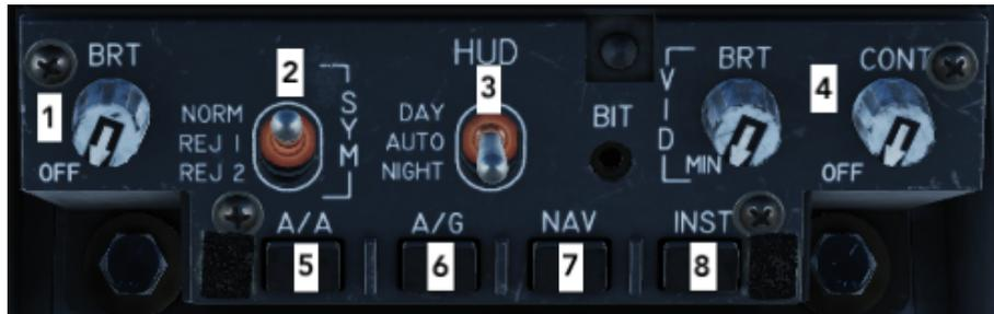
1. Symbol Brightness knob controls the brightness of the HUD stroke symbology. Rotating it clockwise applies power to HUD.
