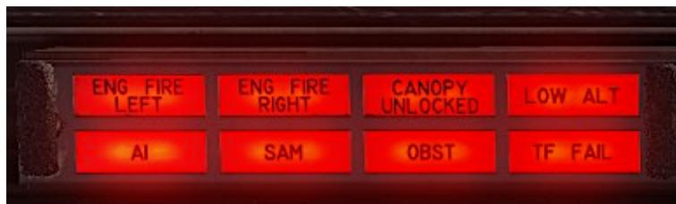
**ENGINE FIRE LEFT** indicates fire condition detected in the left engine. The WSO has no access to fire extinguishing system.
