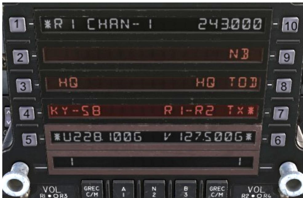
**R1 CHAN - 1 (PB 1):** Indicates the currently selected radio (R1 = UHF, R2 = V/UHF) as well as the preset channel (1 in this case), which can be changed via the scratchpad.
