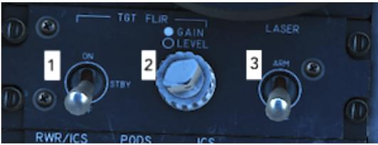
The Sensor Control Panel in the back seat is used for TGP operation.
