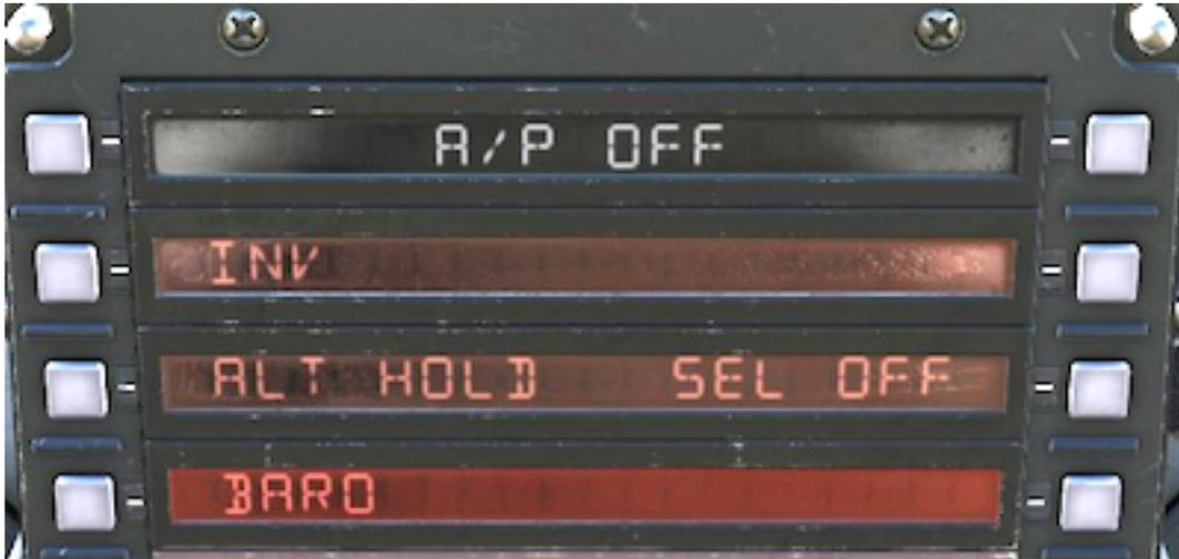
The autopilot submenu provides the means of coupling the current aircraft steer mode and altitude mode. When the autopilot is engaged the autopilot status (same as menu 1) is displayed centered on the top line. If A/P is not engaged, A/P OFF is displayed instead.
