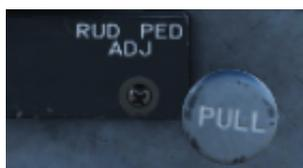
When this knob is pulled, the rudder pedals are released and can be moved back or forward to increase comfort for the operator.
