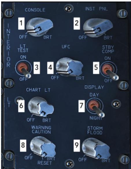
The names of different knobs are mostly self-explanatory and do not need further details. All the knobs offer varied lighting intensity between OFF and BRIGHT.
