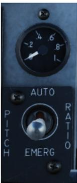
Pitch Ratio Select Switch and Indicator. The switch has two positions: AUTO, which provides normal system functions and EMERG, which removes hydraulic pressure from the hydromechanical pitch control system and causes the pitch ratio and the PTC to drive to a midrange position and lock.
