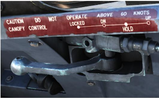
Internal Canopy Control Handles in both cockpits are interconnected to follow each other whenever one handle is moved. There are four positions:
