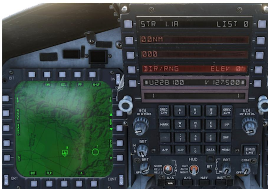
This menu allows the aircrew to create an Offset or Aim Point using range (in NM) and magnetic bearing from the mother Target Point or Steer Point.
