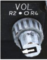
The right Volume Knob controls the volume of the V/UHF radio (R2) with the outer (smaller) knob. The inner (larger) one is not used, as R4 was never added to the F-15E.
