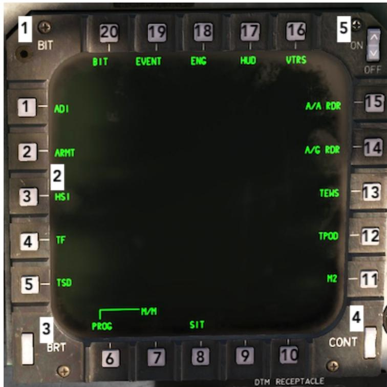
1. BIT Indicator. A magnetically controlled BIT ball rolls over to indicate white when an MPD / MPCD has failed.
