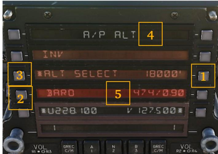
1. First step is to type the desired altitude in the scratchpad and then enter it into the system by pushing PB 8. The altitude value may be between 1000 and 50,000 feet. If the entry is between 10 and 50, it will get multiplied by the system x100.
