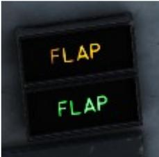
Flap Position Indicator shows the status of the flaps. If the lights are off, that means the flaps are fully retracted. **YELLOW** light indicates that the flaps are in transit. A **GREEN** light indicates that the flaps are down.
