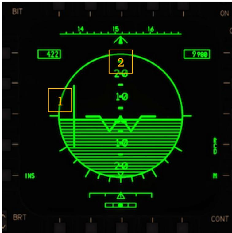
1. On the ADI data from the HUD is mirrored, with vertical Bank Steering Bar.
