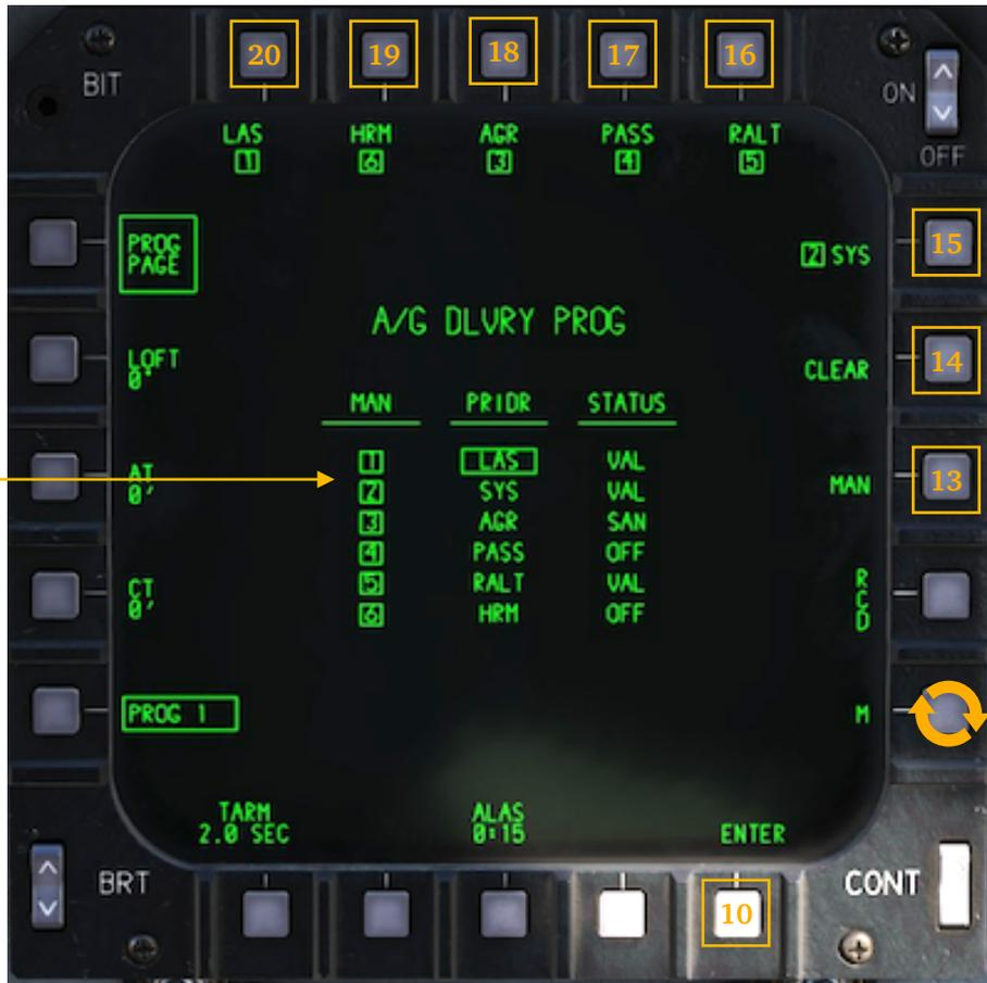
**PB 10, ENTER:** pressing this PB enters the sensors selected at PBs 15 thru to 20 into the manual sensor hierarchy. The selected sensors are then positioned accordingly to the number assigned to each of them (see examples below).
