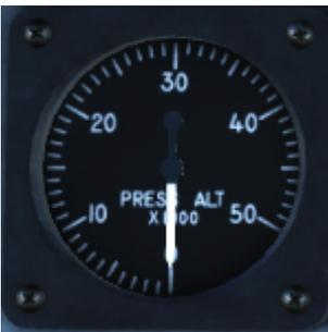
Displays the pressure altitude of the cockpit on a 0-50,000 foot scale. On the ground the displayed value should be equal to the actual field elevation.
