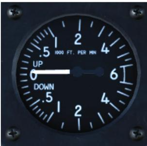
**Vertical Velocity Indicator (VVI)** displays the vertical speed of the aircraft in feet per second (0-1000 in 100 foot marks, then from 1000 to 6000 in 500 foot marks) for both climb and descent. An OFF flag is displayed if electrical power is lost and instrument readouts are not valid.
