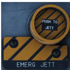
The emergency jettison button is located on the center of the front instrument panel to the left of the MPCD. When pressed, it causes a sequenced jettison of all carted pylons. The button will work as soon as electrical power is on the aircraft, even on the ground. .
