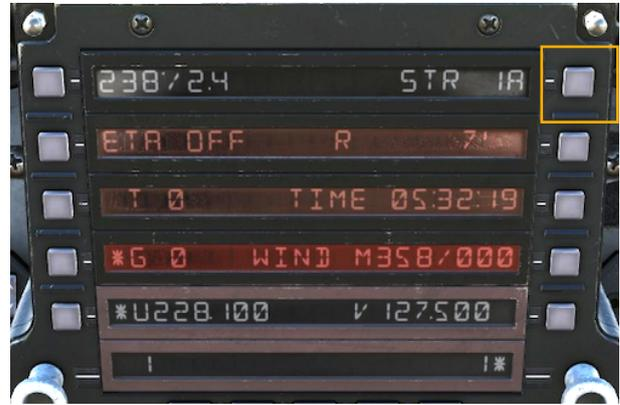
If only a number is typed, the system will select a steer point with a given number within the currently selected route.
