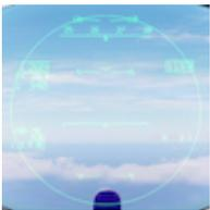
**Supersearch Mode (SS)** scans a 20° by 20° area in 6-bar scan pattern in front of the aircraft up to 10 NM.
