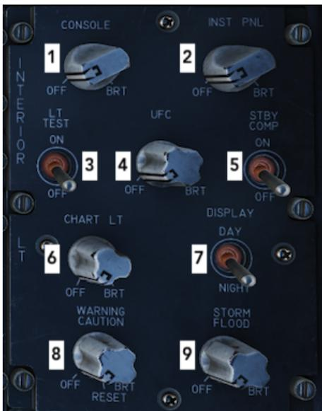
The names of different knobs are mostly self-explanatory and do not need further details. All the knobs offer varied lighting intensity from OFF to BRIGHT.
