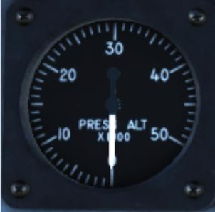
**Cabin Pressure Altimeter** displays the pressure altitude of the cockpit on a 0-50,000 foot scale. On the ground the displayed value should be equal to the actual field elevation.
