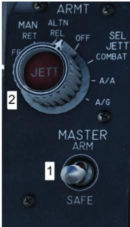
1. Master Arm Switch with two positions. When SAFE is selected, no weapons can be employed. In ARM (up) position, power is applied to the master arm switch, which in turn provides power for weapons release / launch and gun firing.
