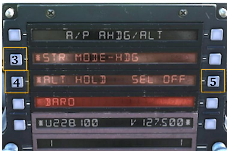
On the UFC, STR MODE-HDG will be shown in second display line, with the asterisk next to it as soon as the A/P button is pressed (3).
