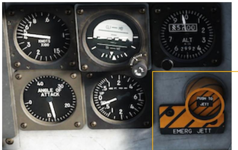
When pressed for approximately 1 second, the contents of all CFT stations and stations 2, 5 and 8 pylons are jettisoned.
