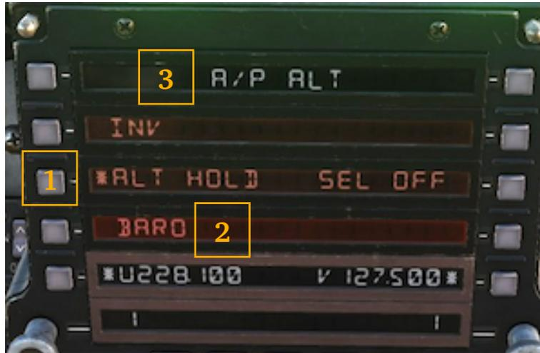
1. In order to enable this mode, ALT HOLD legend has to be marked by pressing the PB 3, which will cause an asterisk to appear next to it. The press of A/P button activates it.
