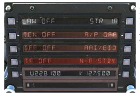
**MENU 1** allows to bring up the Steer Point Menu (PB 10), Auto Pilot Menu (PB 9), Low Altitude Warning (PB 1), TACAN (PB 2) and Terrain Following (PB 4).
