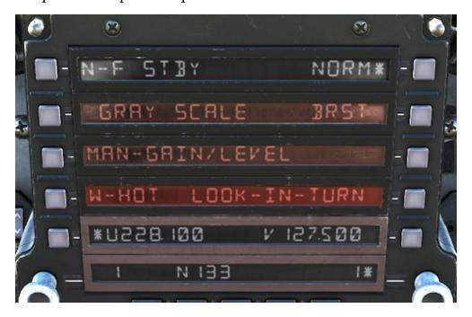
N-F (PB 1): Indicates the current status of the LANTIRN navigation FLIR as described above (OFF, N/R, 5TBY, NORM, BR5T).
