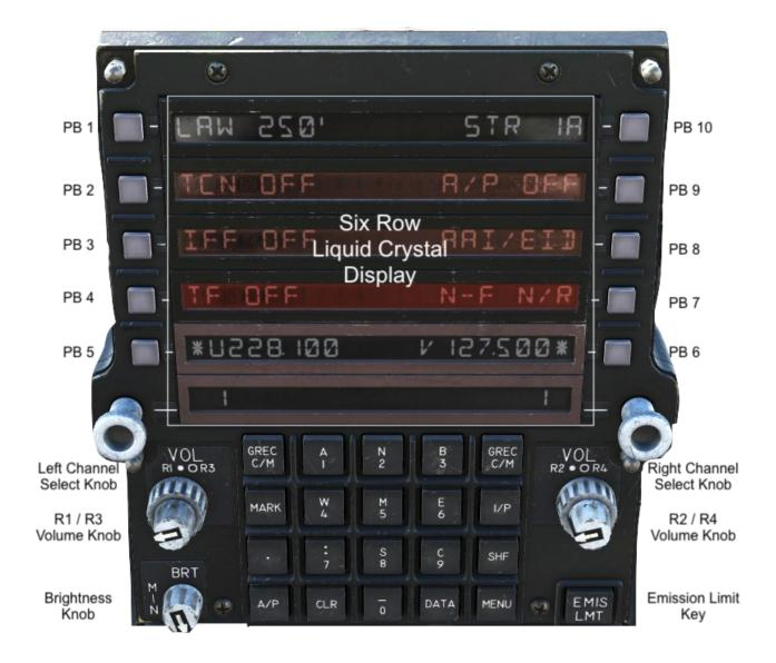
**Six Row Liquid Crystal Display (LCD)** each with maximum 20 characters it can display. Rows 5 and 6 (with brown frame) are exclusively used for the radios. Pushbuttons 1 to 10 (going counter-clockwise from top left to top right) are used to select / interact with menu items displayed in each row.
