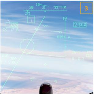
After lockon, the HUD GUNS steering display is provided (3) and the A/A RDR display shows target track data (4).
