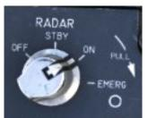
The Radar Power Knob on the sensor control panel has the following functions:
