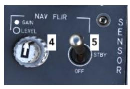
**NAV FLIR Power Switch (5)** needs to be set to ON position for the NAV FLIR option to be used.
