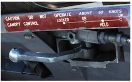
Internal Canopy Control Handles in both cockpits are interconnected to follow each other whenever one handle is moved. There are four positions:
