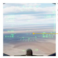
The targeting pod LOS is displayed on the HUD as a segmented box, representing what is displayed on the targeting pod NFOV (1.65°). This symbol is displayed in all Master Modes.
