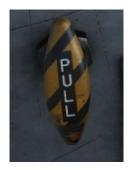
Emergency Landing Gear Handle is used to lower the landing gear bypassing the normal hydraulic and electrical controls. The Emergency Landing Gear Handle in the front cockpit can be reset by rotating the handle 45 degrees clockwise and pushing it forward.
