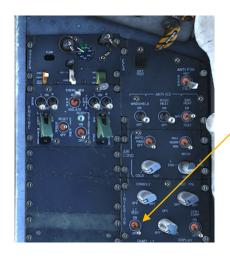
34. Test the cockpit lights and warnings using the LIGHTS TEST SWITCH
