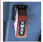
This switch was used in the F-15E with PW-220 engines and has no function with the PW-229.
