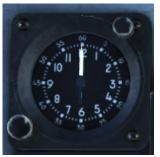
A standard clock with stopwatch function that can be controlled using the pushbutton on the bottom - left. The clock by default is set to display the local time.
