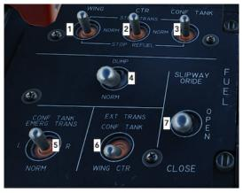
Contains switches governing the fuel system and external tanks. These are:
