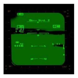
With the N-F boxed, the NAV FLIR image is now displayed on the MPCD or MPD.
