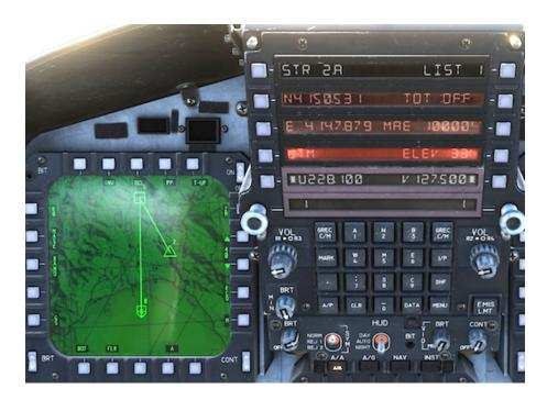
Note that in the example above, the change of SP 2 into a Target Point automatically changed SP 1 into the Ingress Point.
