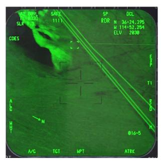
The picture on the left shows the A/G radar in RBM mode. The CUE cursor was selected and spot underneath it was designated (indicated by the EUE legend next to it).
