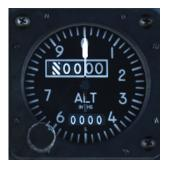
**Standby Altimeter** operates directly from the static pressure source. The rotating pointer shows hundreds of feet. Current altitude is displayed on the dials in the top window, while the bottom one shows currently selected barometric pressure in inches of mercury.
