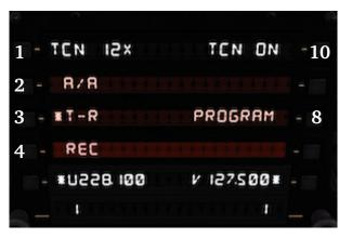
**PB 1:** TCN channel. Pressing this PB switches between X and Y modes.
