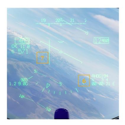
On the HUD, HHD5 legend will also be displayed in the NAV data block to signify that the HDG coupled mode is active (6). A vertical steering line will also be shown (7).
