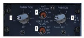
1. Formation Lights Knob control the brightness of six position lights (two on wingtips, one on each side of fuselage forward of the cockpit, one on aft fuselage behind the wing. Available options are OFF, 1-5 (increasing the brightness) and BRT (the full brightness position).
