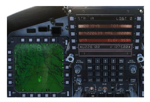
In the example above, there is only one Steer Point (1A) in the current flight plan. To add a new Steer Point, type the number higher than the number of points currently stored in the system and press PB 1 on the UFC.
