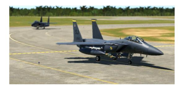
Release the HOLDING BRAKE and enter the runway. Set up in the middle and stop the aircraft by applying and holding the toe brakes.
