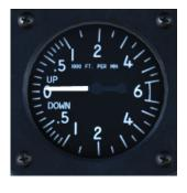
**Vertical Velocity Indicator (VVI)** displays the vertical speed of the aircraft in feet per second (0-1000 in 100 feet marks, then from 1000 to 6000 in 500 feet marks) for both climb and descent. An OFF flag is displayed if electrical power is lost and instrument readouts are not valid.
