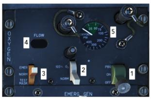
Control panel for the Molecular Sieve Oxygen Generating System (MSOGS). The MSOGS provides a continuously available supply of breathing gas for the aircrew.
