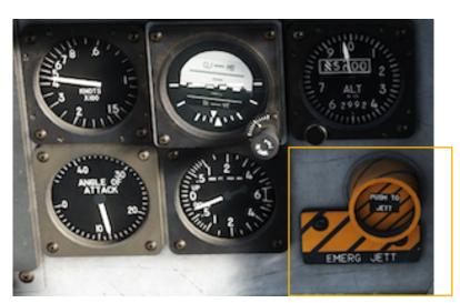
When pressed for approximately 1 second, the contents of all CFT stations and stations 2, 5 and 8 pylons are jettisoned.
