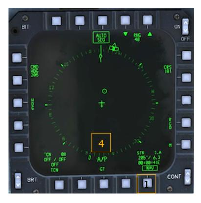
Second line of display on the UFC will show 5TR MODE-NAV legend with an asterisk next to it (2). When the A/P button is pushed on the UFC, A/P NAV shows in the first line of display (3), with additional A/P information on the HSI (4).
