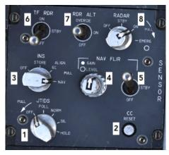
Contains switches for different onboard sensors and systems, such as radar, NAV FLIR and INS.
