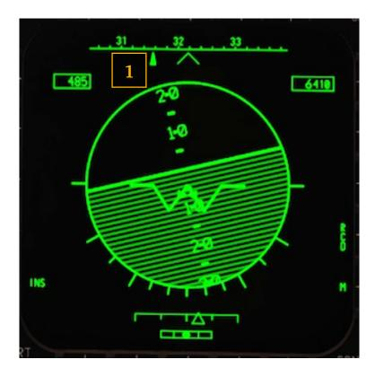
1. Information on the ADI largely mirrors the one shown on the HUD, with Command Heading displayed on the heading scale.
