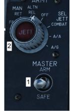
**1.**Master Arm Switch with two positions. When SAFE is selected, no weapons can be employed. In ARM (up) position, power is applied to the master arm switch, which in turn provides power for weapons release / launch and gun firing.
