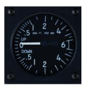
**Velocity Vector Indicator (VVI)** displays the vertical speed of the aircraft in feet per second (10-100 in 10 feet marks, then from 100 to 600 in 50 feet marks) for both climb and descent. An OFF flag is displayed if electrical power is lost and instrument readouts are not valid.
