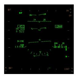
The HUD repeater can be enabled on any MPCD / MPD in front or rear cockpit.
