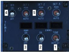
The TEWS is an integrated suite consisting of four subsystems: Radar Warning Receiver (RWR), the Internal Countermeasures Set (ICS), the Electronic Warfare Warning Set (EWWS), and the Countermeasures Dispenser (CMD) Set.
