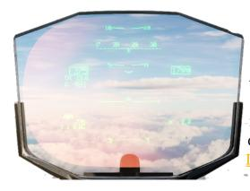
The holographic combiner displays projected raster (video) and stroke (symbols) imagery in a total field of view which measures 21° in elevation and 28° in azimuth. The HUD displays navigation, FLIR video, flight control and weapon delivery information. See <a href="Chapter 6">Chapter 6</a>: Head Up <a href="Display">Display</a> for more information.
