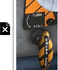
The emergency vent handle electrically dumps cabin pressure when turned 45 degrees counterclockwise. When extended, it shuts off ECS air to the cockpit and allows ram air to enter.
