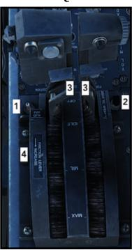
The front throttle quadrant contains the front throttles, finger lifts, friction adjusting lever, rudder trim switch and flap switch. Additionally, the throttle grips contain switches to provide various system controls without moving the left hand from the grips.
