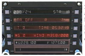
**DATA 1** is used mostly for information purposes and provides crew members with intel about bearing and distance (PB 1) to current steer point (PB 10), estimated time of arrival or time to go (PB 2), selection between True (PB 3) and Ground (PB 4) speed and current winds.
