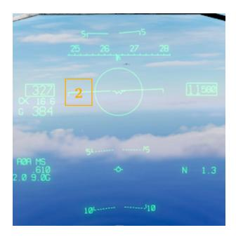
On the radar display, B5T legend in the bottom - left part (1) indicates that the radar is in Boresight mode. On the HUD, target should be placed in the scan circle to achieve an automatic lockon (2), upon which the radar enters normal STT.
