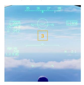
On the radar display, LR B5T is displayed in the bottom - left part (1). The range of the scan is set to 40 NM (2). On the HUD, target should be placed in the scan circle to achieve an automatic lockon (3), upon which the radar enters normal STT.
