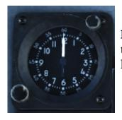
**Eight Day Clock is** a standard clock with stopwatch function that can be controlled using the pushbutton on the bottom - left. The clock by default is set to display the local time.
