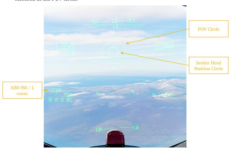
**FOV (FIELD OF VIEW) CIRCLE** remains centered on the HUD. It is removed when the seeker is uncaged and tracking target or when radar is in angle track.
