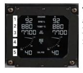
This display is the primary source of engine data, although additional information can be found on the MPD / MPCD in Engine menu. The data displayed for the Left and Right engine is as follows:
