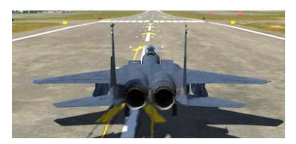
Advance engines to 82% and check the instruments and caution / warning lights. When ready for takeoff, release brakes and advanced the throttles to MIL or MAX power (as desired).
