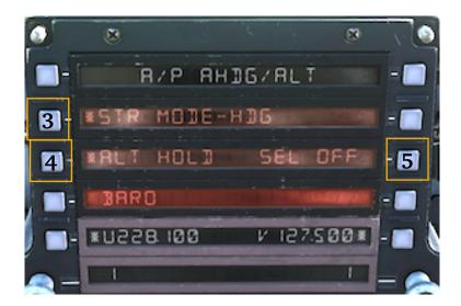
On the UFC, 5TR MODE-HDG will be shown in second display line, with the asterisk next to it as soon as the A/P button is pressed (3).
