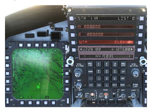
It is possible to create Offset / Aim Points by entering the Lat - Long or UTM coordinates in exactly the same way as for the Steer Points. However, there is additional option available after pressing the PB 4 when in UTM sub-menu (marked RNE / BRE):
