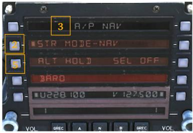
The aircraft will now turn to intercept the currently selected Sequence Point. It will maintain the pitch angle the aircraft had when the autopilot was engaged.
