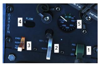
Control panel for the Molecular Sieve Oxygen Generating System (MSOGS) is exactly the same in the back seat as in the front. The MSOGS provides a continuously available supply of breathing gas for the aircrew.
