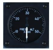
**Cabin Pressure Altimeter** displays the pressure altitude of the cockpit on a 0-50,000 foot scale. On the ground the displayed value should be equal to the actual field elevation.
