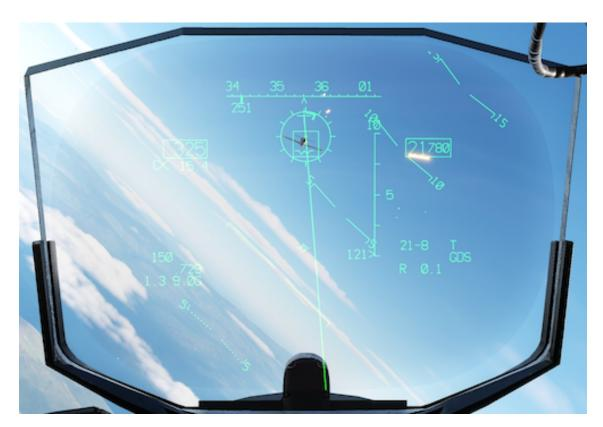
Even though in theory the reticle should be aligned with the gun cross, the bullets are flying to where the gun cross is pointing, so above the target.
