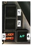
When the laser is armed, appropriate red warning light will be visible on the top-left caution lights panel (3) in the front cockpit.
