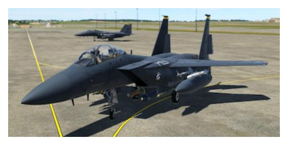
Advance the throttle enough to start moving again and taxi via the assigned taxiways to the designated runway. During taxi, check all the flight instruments. At high gross weights, make sure to perform all turns at minimum practicable speeds and maximum practicable radius. At low gross weight, closely monitor your taxi speed, as there may be excess thrust at idle throttle position.
