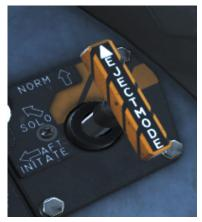
Available only in the rear cockpit, allows operator to select the desired ejection sequence to be initiated from the rear cockpit, or provide for single ejection for solo flight. Positioning is accomplished by pulling full aft then turning to the desired position.
