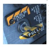
When pulled, this handle provides additional power from JFS hydraulic accumulator to the brake system and for the nose gear steering. In case of brakes failure, sufficient power is provided to safely stop the aircraft.
