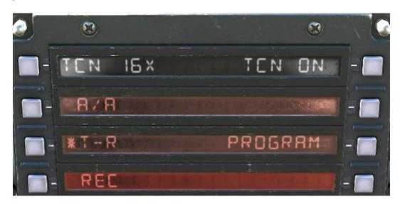
Pressing the PB 8 (PROGRAM) opens another page which allows to enter additional data for the TACAN station.
