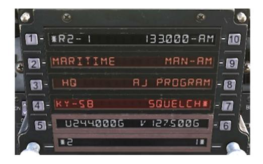
**R2 - 1 (PB 1)**: Indicates the currently selected radio (R1 = UHF, R2 = V/UHF) as well as the preset channel (1 in this case), which can be changed via the scratchpad.
