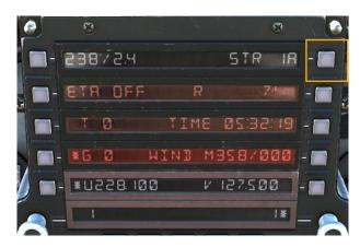
If only a number is typed, the system will select a steer point with a given number within the currently selected route.
