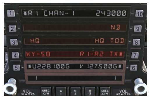
**R1 CHAN - 1 (PB 1)**: Indicates the currently selected radio (R1 = UHF, R2 = V/UHF) as well as the preset channel (1 in this case), which can be changed via the scratchpad.
